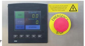
The touch screen HMI can be programmed to show and control belt speed and lamp intensity or configured to customer specification
